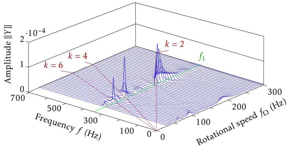
Figure 1.4: Spectrum of the rod's response
