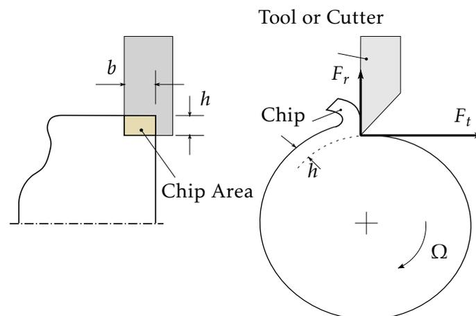
Figure 2.1: Cutting process in turning; constant chip width
