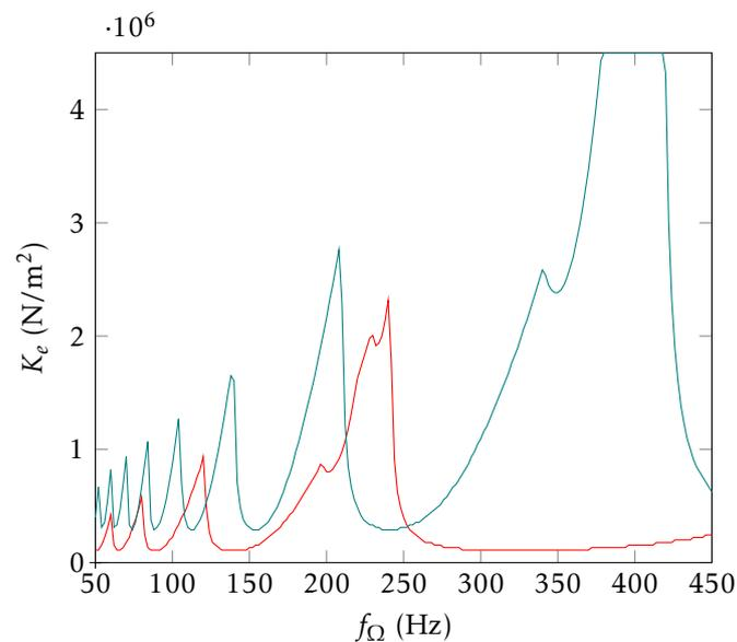
**Figure 4.7:** Influence of the rod's stiffness:  $\alpha = 0.5$  (—),  $\alpha = 1.5$  (—)
