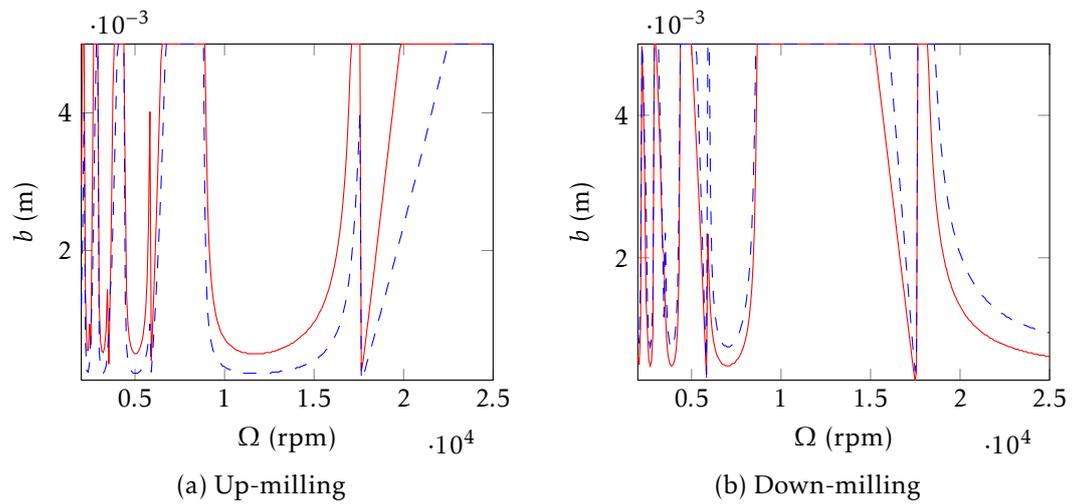
Figure 3.2: SLD Milling 1DoF: Chebyshev Collocation (—), SDM (---)
