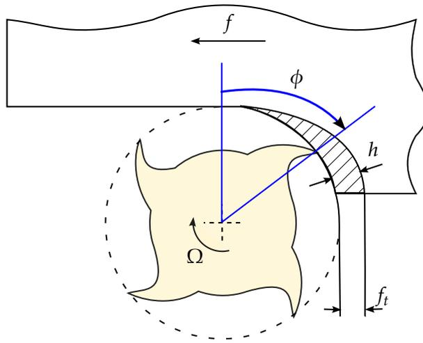
Figure 2.2: Cutting process in milling & periodic chip variation
