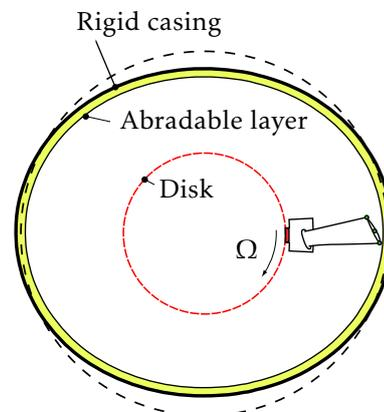
Figure 1: Casing shape [24]
