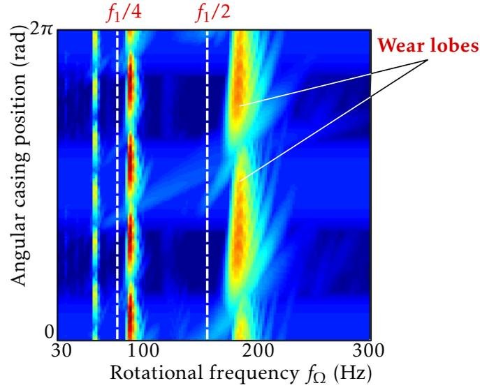
Figure 1.3: Abradable layer profile after 20 revolutions
