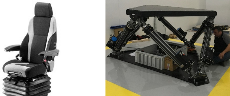
Figure 1 – Example of (a) a suspension seat and (b) a multi-axis platform for vibratory characterization
